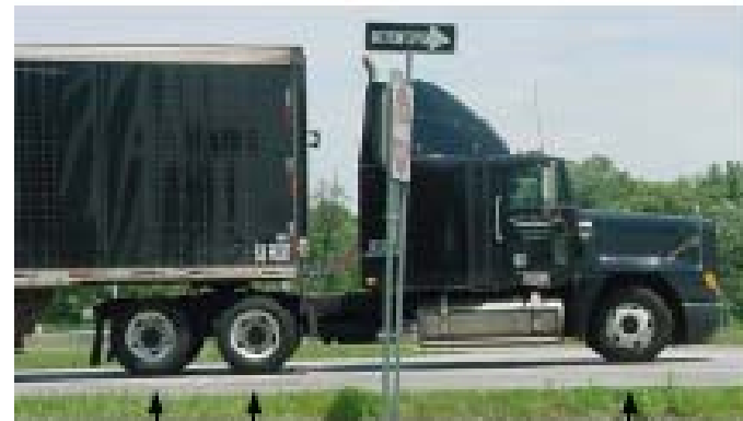
Rear Drive Tandem Axle (Axle 3)
